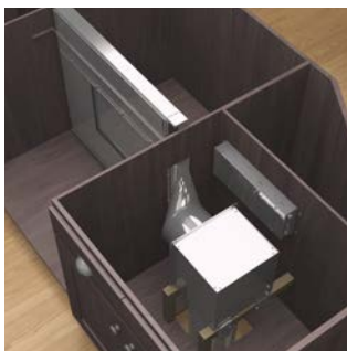
In-cabinet blower placement, left or right side.
