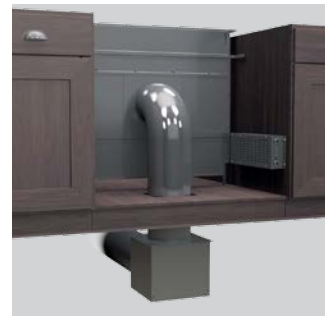
Duct transition in front of downdraft to blower installed below the floor line.
